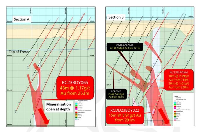
Figure 5 | Typical Cross section of Neptune prospect showing wide, high-grade zones of continuous mineralisation, with existing drilling limited to ~80m depth
